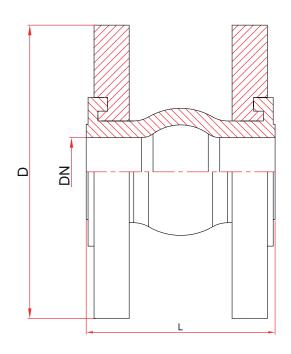
Expansion: Axial + 15mm - 20 mm Radial 15 mm
